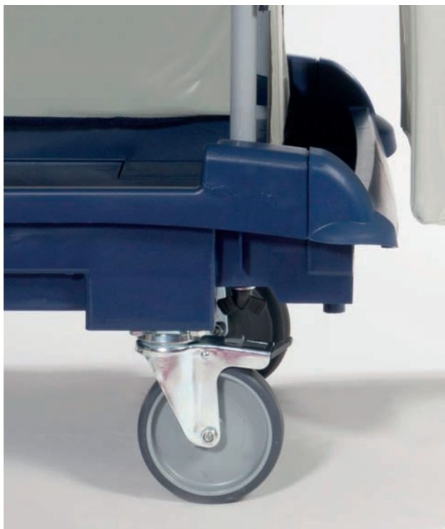
Castors fixing. The wheels are applied with a four point fixing support firmly held between the base and a stainless steel plate with thickness 1,5 mm.
