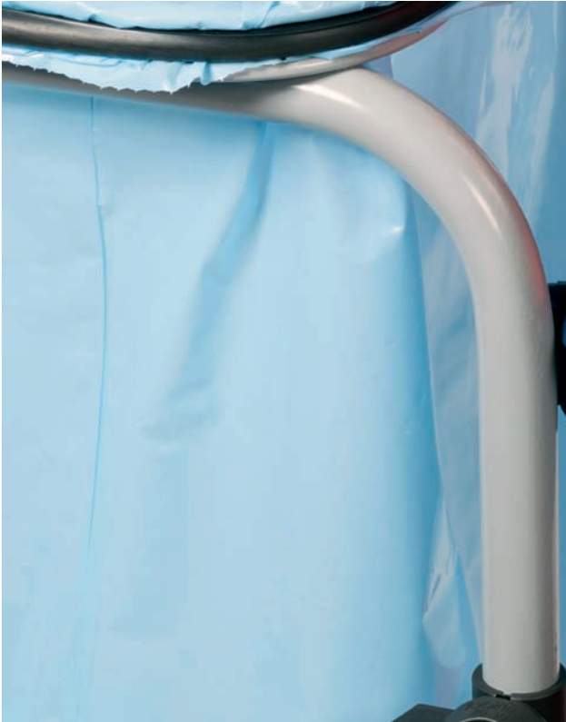
VDM Rilsan protection. VDM exclusive excellence is the special Rilsan protection by immersion in fluid bed (protective film thickness 400 micron) which grants a high duration over the time.
